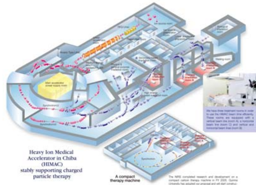
Fig. 4 Schematic overview of HIMAC with its three cancer treatment rooms and a new compact therapy machine
