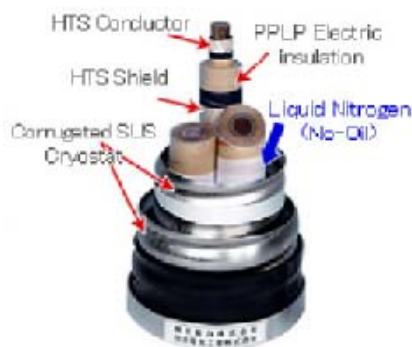
Fig. 5: high- T_c superconductor (HTS) cable cooled with liquid nitrogen (from http://global-sei.com/super/cable_e/index.html )
