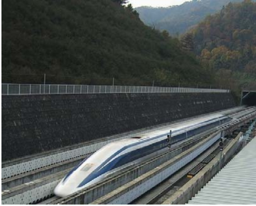
Fig. 2: maglev train MLX01-2 at JR's Yamanashi test track which has recorded the highest speed of 581 km/h (from Wikipedia)
